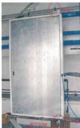
Photo 3: Test set-up for measurement of Weatherseal gap.
